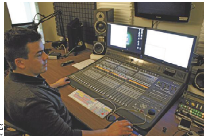
The mixing room equipped with a ProTools HD, Media Composer Video Satellite and C24 control surface.
